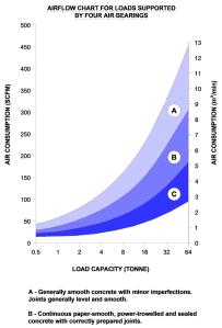
C - Continuous self-levelling epoxy or joint free steel sheet.
